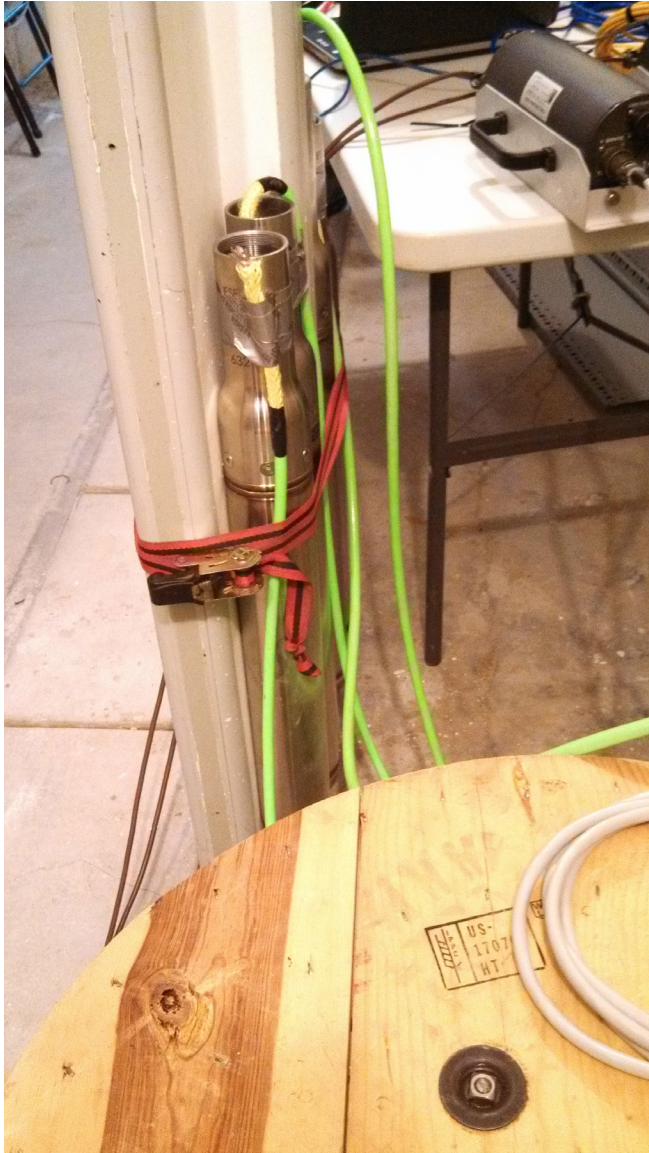
Figure 4.5.3: The first geophone test in Byerly Vault, January 2014. The geophone borehole packages were strapped to the support between two instrument bays during the test.
